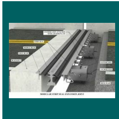
3 Inch Strip Seal Expansion Joint
